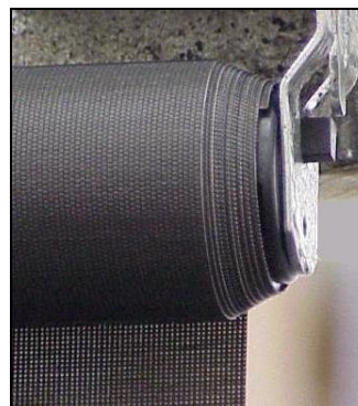
Figure 12 Telescoping to the left
